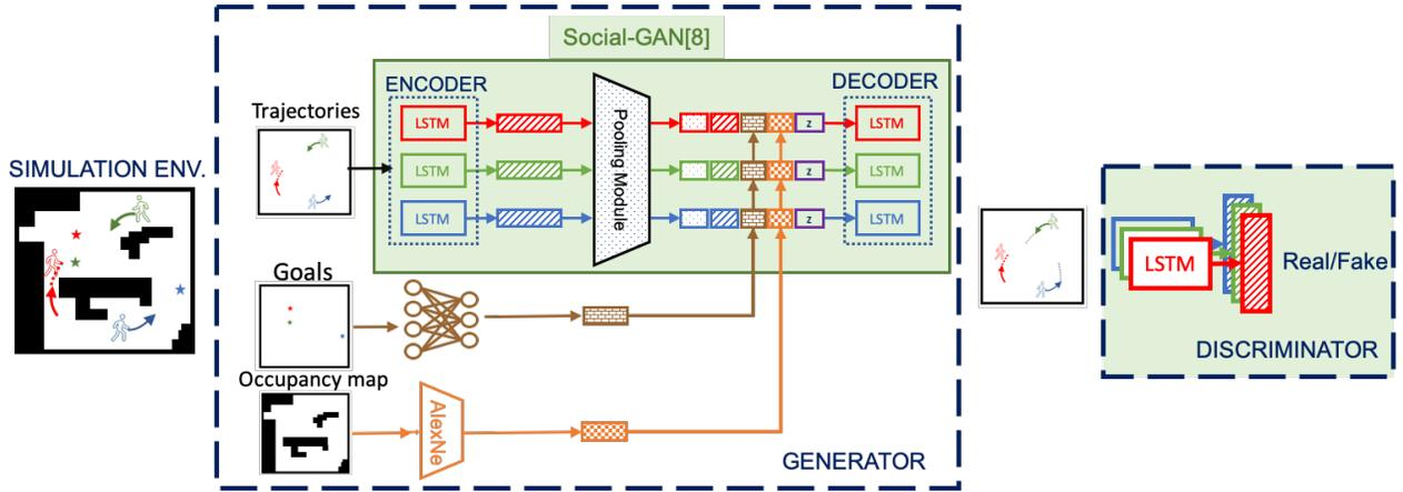
Fig. 3: Proposed model. We use the GAN-based encoder-decoder structure and pooling layer from Social GAN [8] as our backbone model, and incorporate the knowledge of pedestrian short-term goal positions and local obstacles so that the local controller can better follow the global plan while avoiding local collisions.
