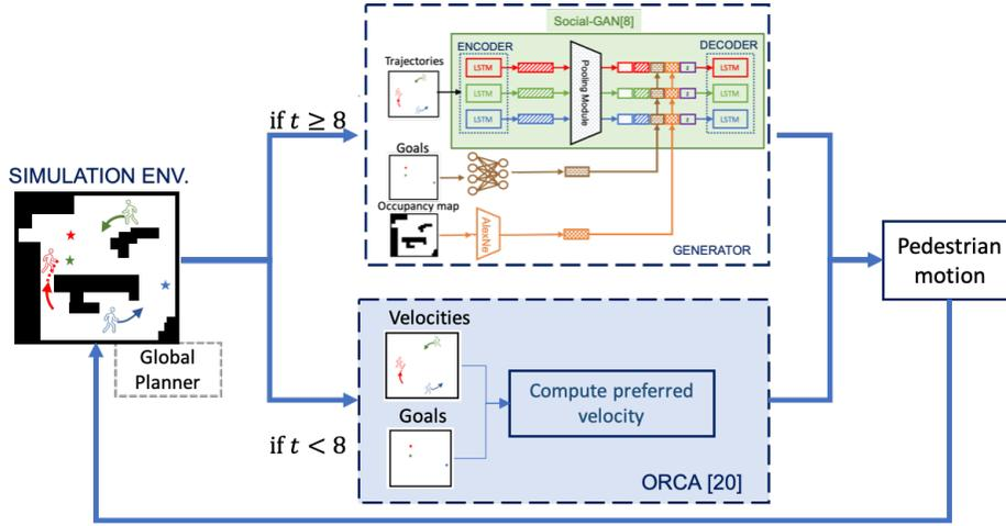
Fig. 2: Overview of our pedestrian simulation pipeline. The iGibson global planner creates a set of waypoints that the local planner uses as short-term goals. The local planner also takes the occupancy map of iGibson’s indoor environment and trajectory histories of each pedestrians as input and predicts the next positions for each pedestrian. The trajectory history is initialized by running the default ORCA simulator for first 7 time steps (i.e.  $t < 8$ ) of each episodes.
